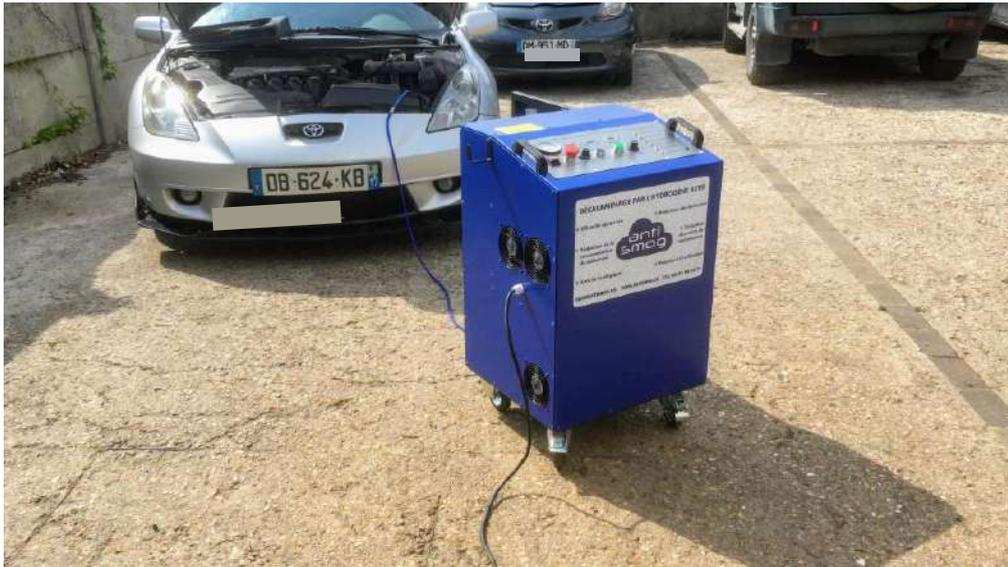
A typical setup for carbon-cleaning of a car
