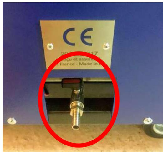
Drain valve at the back of the machine
