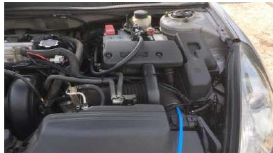
Hydrogen delivery hose placement in the air admission duct
